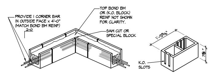
"KNOCKOUT" OF TROUGH BOND BM BLOCK (TYPICAL UNIT EXCEPT @ ALL OPNGS; SOLID BOT BD. BM SHALL BE USED. PROVIDE GROUT STOP (RE:SPECS.) UNDER K.O. BOND BEAMS OVER CELLS WHICH ARE NOT TO BE REINFORCED AND GROUTED.
