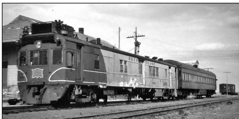
Left: A rare EMC-AB6 manufactured expressly for the Rock Island by the Electro-Motive Corporation (EMC) was capable of pulling additional cars. This Doodlebug ran between Eldon and St. Louis until 1959.
