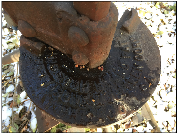
Switch track lever and detail of manufacturer markings on this structure.
